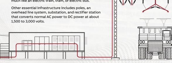
Because of the high power requirements of the trolley system, the operator may also have to increase the site's power capabilities. Using a trolley-assist system on a diesel-electric truck can lead to a substantial reduction in operating costs, with the exact extent dependent on the mine design. The main factors include:
